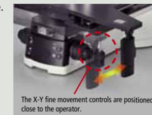
The X-Y fine movement controls are positioned close to the operator.
