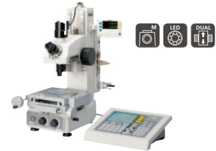
MM-200 with Monocular Eyepiece Tube and DP-E1
