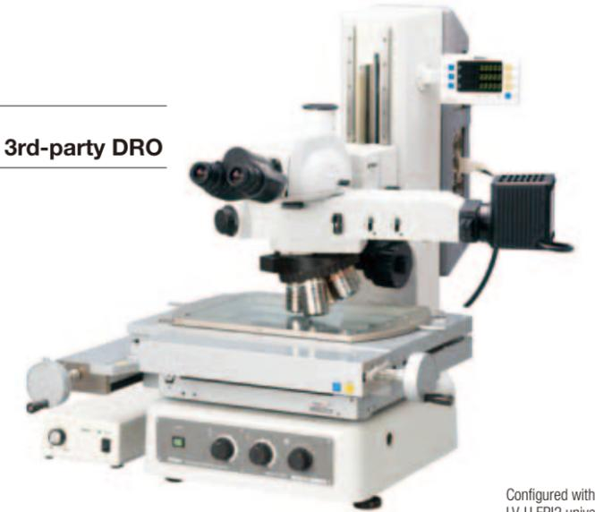
Configured with PS 12x8C stage, LV-U EPI2 universal epi-illuminator, tilting trinocular eyepiece tube with built-in reticle
