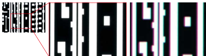
Apochromat optics (captured with SMZ1270+Plan Apo 1x/WF)
