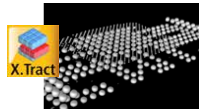
High magnification of BGAs, visualized in a 3D representation
