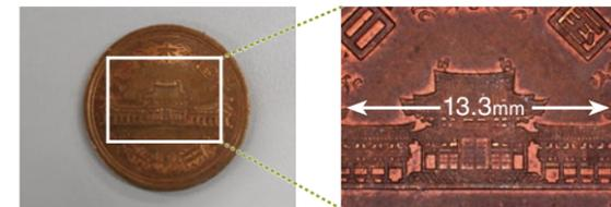
10 yen coin Under coaxial top light at 0.35x optical magnification
