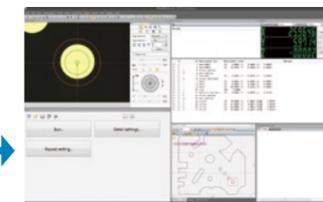
Various wizards for guiding procedures of measurements are available, providing fast, easy writing of teaching files. GUI can be customized for different tasks. You can select and hide functions for achieving your tasks.
