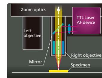
TTL Laser AF schematic
