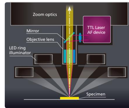
TTL Laser AF schematic
