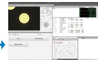
Various wizards for guiding procedures of measurements are available, providing fast, easy writing of teaching files. GUI can be customized for different tasks. You can select and hide functions for achieving your tasks.
