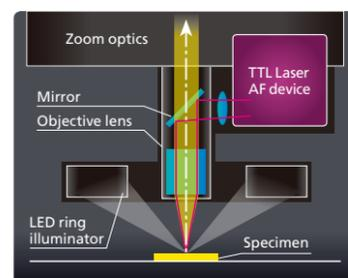
TTL Laser AF schematic
