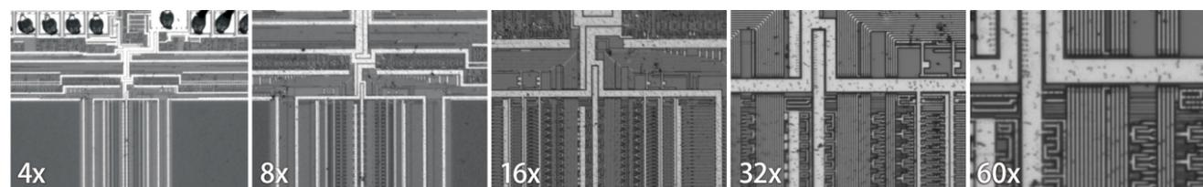
Type 4, having a 4 to 60x optical magnification, twice the magnification of the Type 3, is designed for tiny features in high density specimen. Its objective lens is newly designed with a high N.A. 0.46 and a long working distance 30mm.
