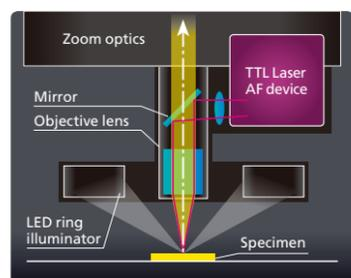
TTL Laser AF schematic
