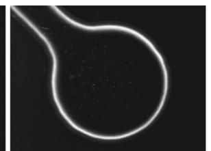
High density PCB Under dark field illumination at optical magnification 16x
