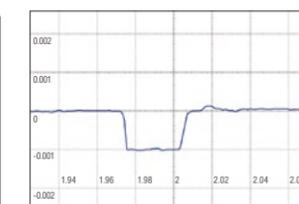
Cross section of a small groove
