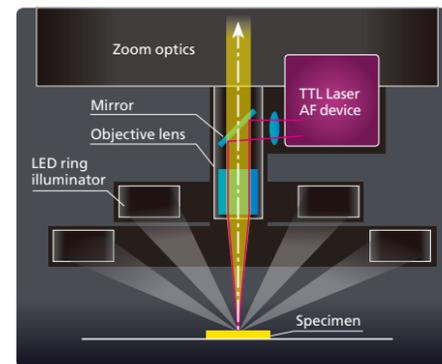
TTL Laser AF schematic
